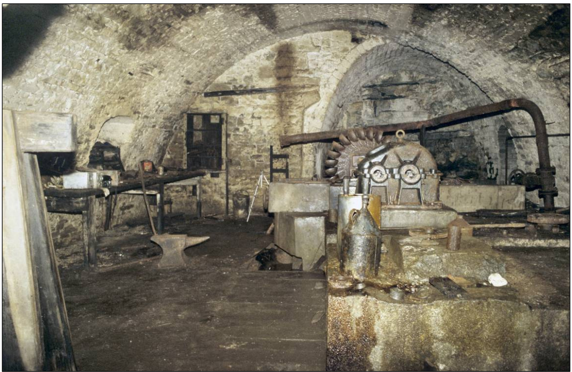
Plate 3: The machinery room at the base of Brewery Shaft - the tools and machinery survive as left nearly 100 years ago. A Pelton wheel is visible right of centre of the photograph.
