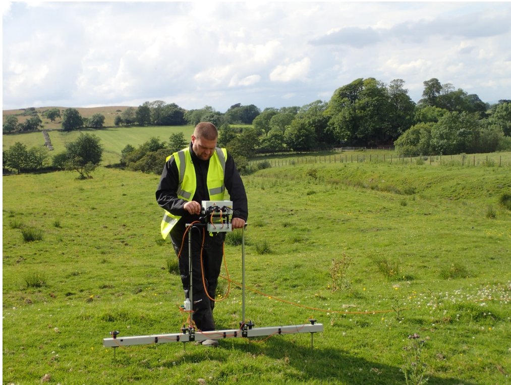
Resistance survey. Hadrian's Wall is visible to rear left, northern ditch to right.
