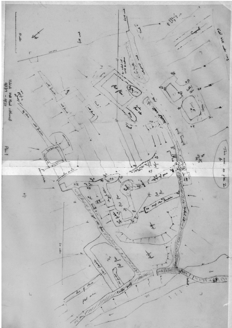
Figure 7: Theodolite and disto survey of core area of Well Head settlement: raw plans. These are the two overlapping plans produced on site. They were checked on site for accuracy and to have hachures and other annotations added. A cleaned-up version is shown in the next figure. Height measurements, measured by a dumpy level, are included on these plans.
